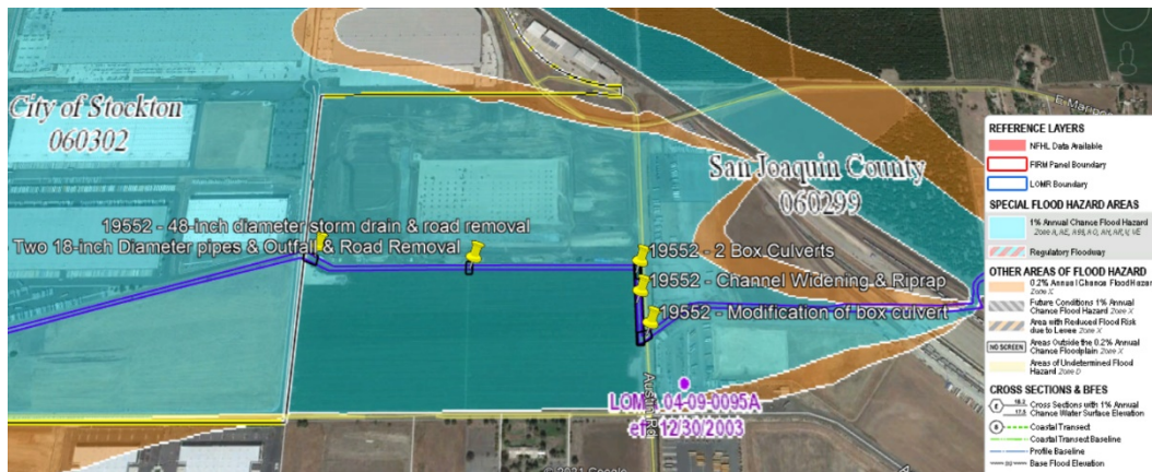
Figure 2. Proposed alterations overlaid onto the FEMA base floodplain map.
